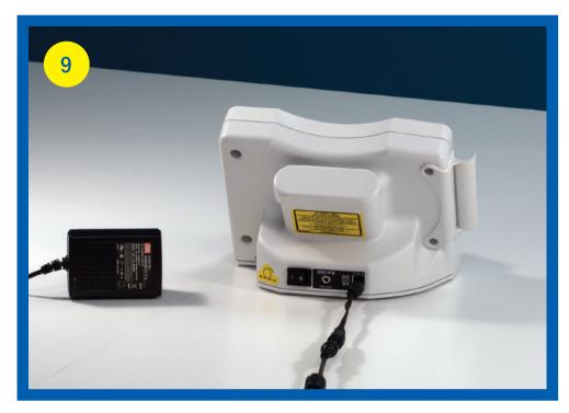
If the battery has 2 bars or less, connect the charger. Do not use the unit with the charger attached.
