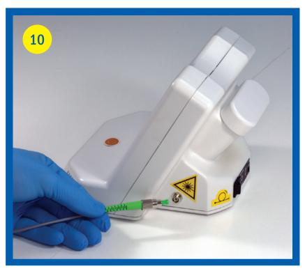
Remove the protective cap from the handpiece and firmly insert all the way in the unit.
