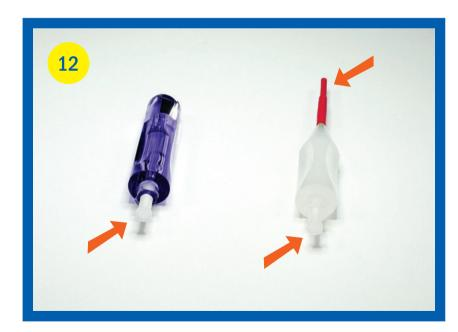
Choose the Laser Tip and remove the plastic plugs, then thread on the handpiece.
