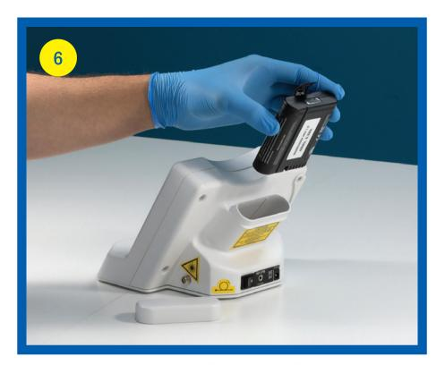
Install the battery inside the unit. If the battery is fully charged, there is no need to connect the power supply.
