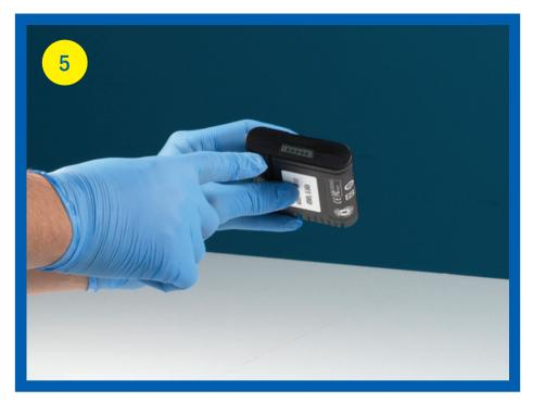
Remove the battery unit from the accessories and check its charge level.
